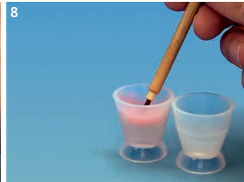
7 The moist brush tip is dipped 3 - 4 mm into the powder.
