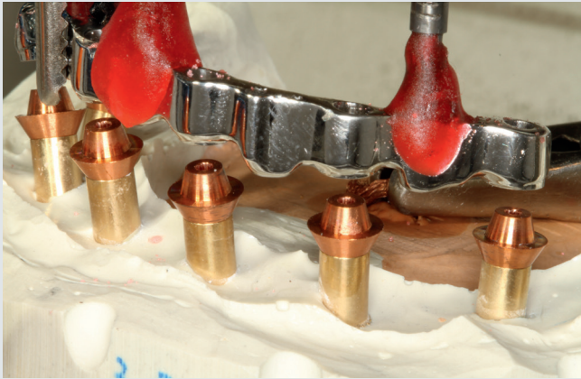
The SAE spark erosion process with electrodes
