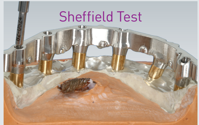
After passivation using SAE spark erosion
