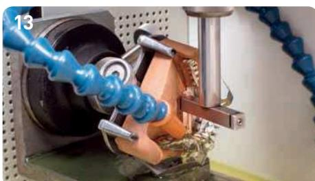
13 The influx of dielectric fluid is commenced, the tank is filled, the spark erosion process begins. For the erosion parameters, see parameter list EDM 2000.
