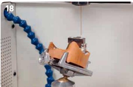
Using forcible control, the electrode (Order No. 30-1004) was lowered into the exact position in the Teflon bushing. The bushing fits an 0.8 mm electrode.
