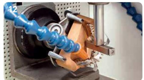
12 The hose for flushing dielectric fluid is positioned at just under 45° to the erosion area.
