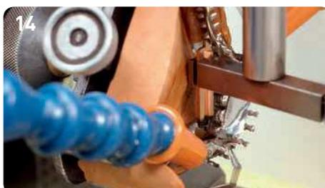
14 The burnt-down electrode following the spark erosion process.
