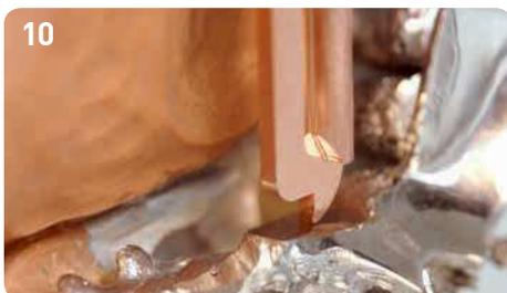
10 The clasp secures the secondary part on the primary part and thus creates the electrical contact. Allow the electrode to slowly move towards the model cast (beep) and then set the depth on the display (depth: 5.5 – 5.7 mm).
