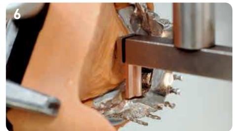
5 Position the model with the primary and secondary parts at a 90° angle to the oral surface. Align the erosion position with the aid of a straight, cut-to-length electrode. Set zero points on display for the X and Y axes.
