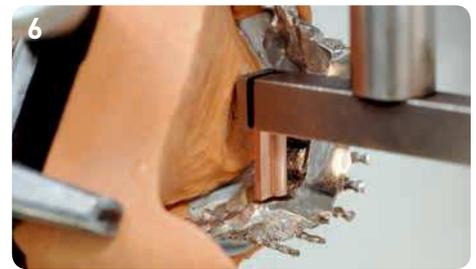
5 Position the model with the primary and secondary parts at a 90° angle to the oral surface. Align the erosion position with the aid of a straight, cut-to-length electrode. Set zero points on display for the X and Y axes.
