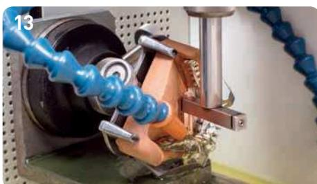
13 The influx of dielectric fluid is commencing, the tank is filled, the spark erosion process begins. For the erosion parameters, see parameter list EDM 2000.
