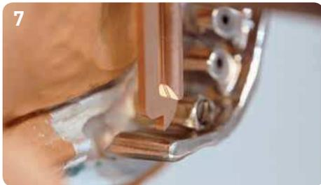
7 Visual control of the electrode position. The electrode should be lowered towards the cone so that the latch nose slots completely into the eroded groove of the tapered cone.
