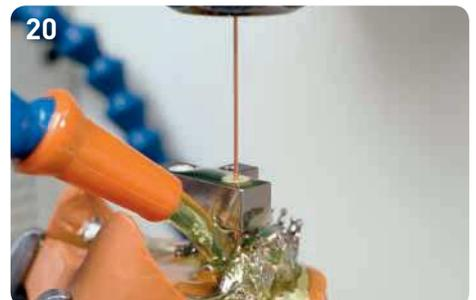
After the influx of dielectric fluid has begun, the erosion process can start – see data sheets for parameters.
