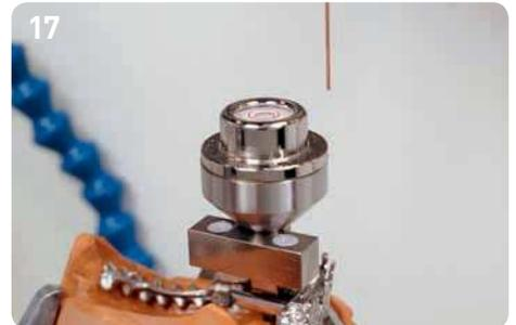
For the erosion of the latch axle at a 90° angle to the eroded latch fit, the latch part (Order No. 30-1242) is inserted into the latch fitting and attached to the axle location (Order No. 30-1602). The spirit level (Order No. 82-1201) inserted into the latch area serves to ensure parallel alignment.
